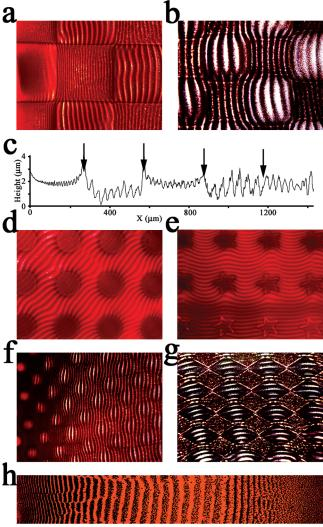
**Figure 3.** Periodic precipitation strucutres on photopatterned gels. (a) UV exposure 810 mJ/cm². Panel c is a profile of a. (b and d-f) UV exposure 300 mJ/cm². (g) UV exposure > 1500 mJ/cm². (h) PP pattern exhibiting both positive and negative values of the spacing coefficient, p. The left half of the pattern developed for 2 h in the dark; the right half, in the light for 4 h afterward.
